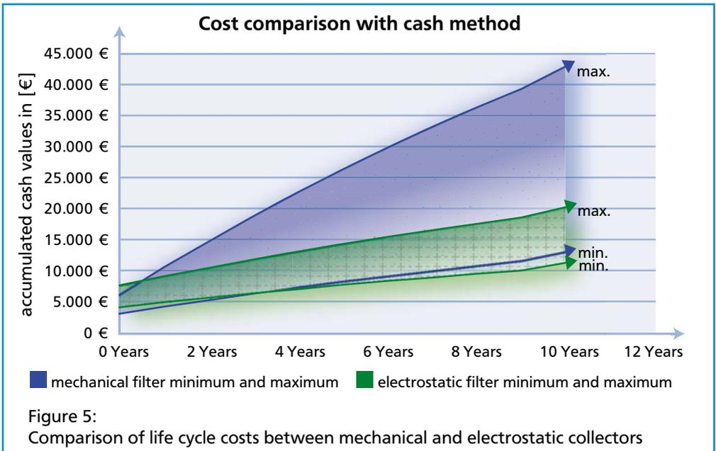
After an operation of 10 years, cost differentials of up to 25,000 € per filter will result – without impairment of air quality. On the contrary: The economy of electricity will reduce CO<sub>2</sub> emissions by at least 2 tons CO<sub>2</sub> per year.
