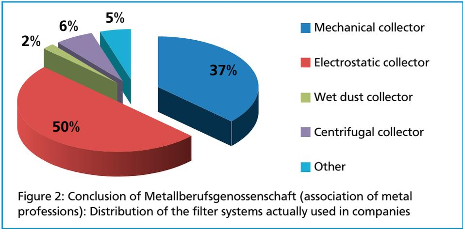
This article considers the life cycle costs for mechanical and electrostatic collectors, only, because in the companies' practise these collectors have a market share of 90% for exhaustion of cooling lubricants; see figure 2.<sup>[2]</sup>
